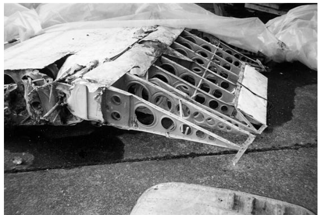
Fabric deteriorated but otherwise sound vertical stabilizer
