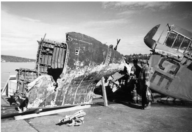
Rear fuselage section - top portion separated during lifting
